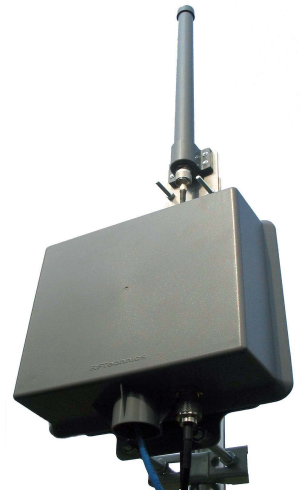
RFT-Link connected to an external omnidirectional antenna. (Access Point)
